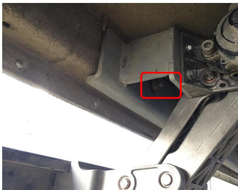
As seen in the picture, the front connection bolts of the carrier chassis are mounted to the vehicle.
