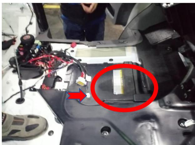
Wiring connections are made to the vehicle's battery.
