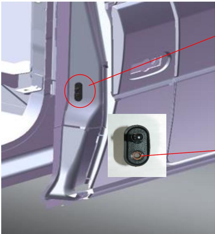
Ø 11 mm hole is drilled for switch assembly.
