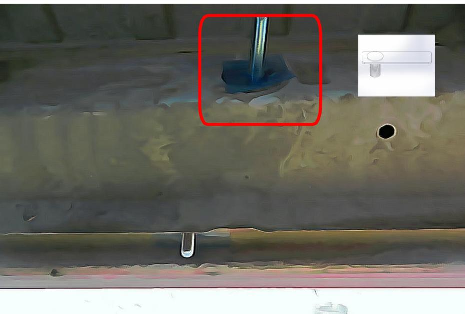
For the carrier chassis connection, 4 bolts are placed in the original chassis holes of the vehicle.
